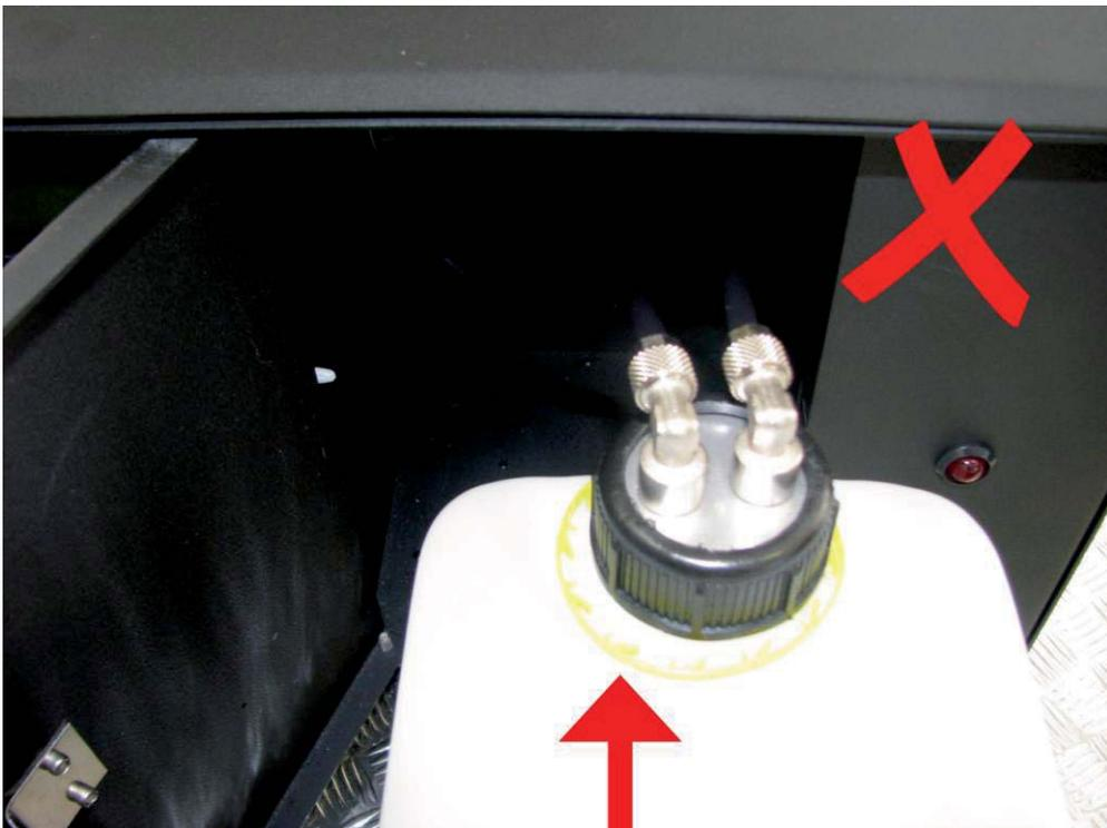
When placing the fluid can into the FLAMANIAC like this, the fluid hose will fold. A folded hose will cause damage to the pump of the unit.
