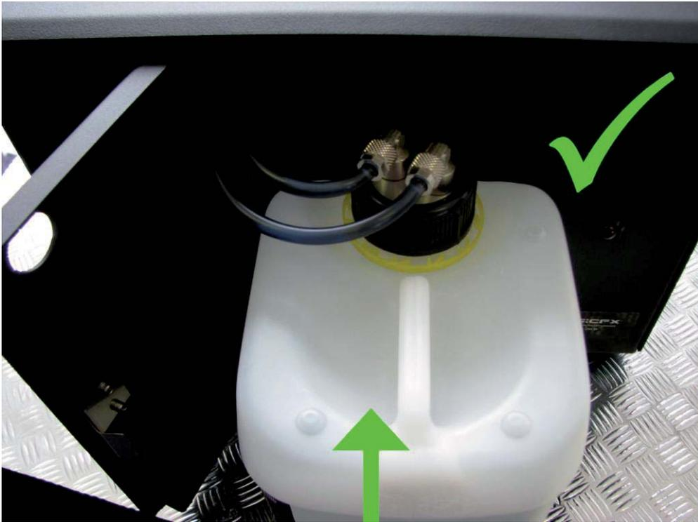
Make sure the can will be inserted like above picture with the fluid hose in a smooth curve.
